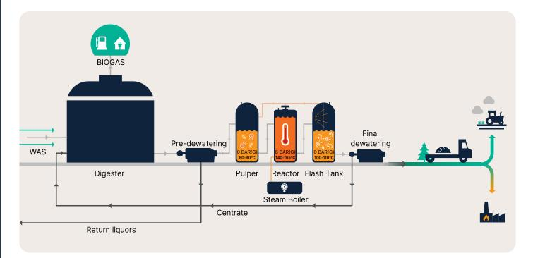
SolidStream is a novel process technology and service, building on Cambi's well known, compact, modular thermal hydrolysis process (THP). Developed in 2013, it is tailored to dramatically reduce sludge handling and disposal costs for wastewater treatment plants (WWTPs) with sufficient digester capacity at existing anaerobic digestion plants.
