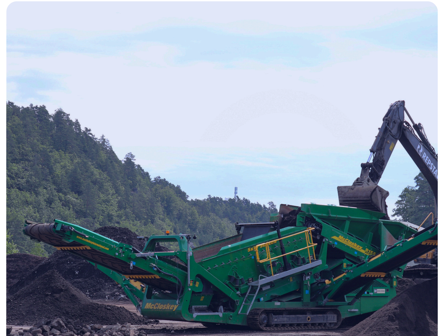
Bulk soil screener at Grønn Vekst's soil production site in Kristiansand, Norway
